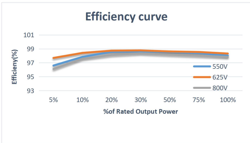
Figure 2-8 Power efficiency curve (take 80KW for example)
